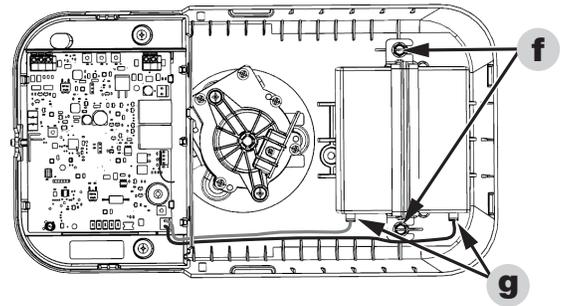
h) Remove the bracket with one hand while securing the battery with the other hand.
